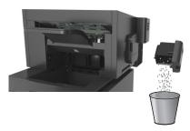
**3** Insert the emptied hole punch box back into the finisher until it *clicks* into place.
